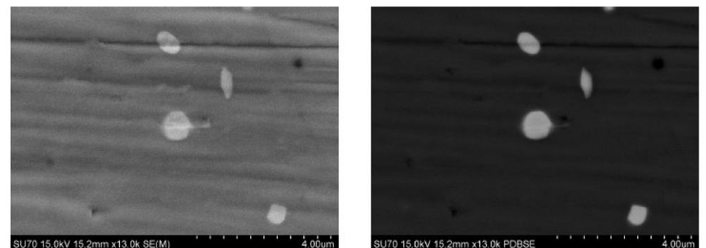
Figure 2. SEM images using (left) SE detectors and (right) BSE detector on a transition metal containing a lanthanide metal. The lanthanide is heavier, and therefore the contrast is stronger in BSE mode. Material is courtesy of Dr Tofail Syed
