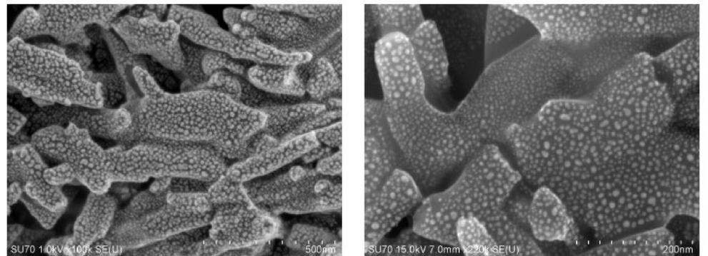
Figure 1. Images of gold islands on conducting film using the upper SE detector at (left) 1kV and (right) 15kV. The resolution remains similar indicating that using the lower voltages for uncoated beam sensitive materials can be done without loss in resolution
