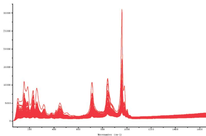
Figure 1: Mapping results of spectra collected in an area of  $10\mu\text{m} \times 20\mu\text{m}$  on the surface of a powder particle of a catalyst. (Mo V6:1, supported by wet impregnation of alumina, previously calcined at  $1150^{\circ}\text{C}$ ). These spectra illustrate the compositional variations e.g.  $\text{V}_2\text{O}_5$  species, MoO (both tetrahedral and octahedral species).
