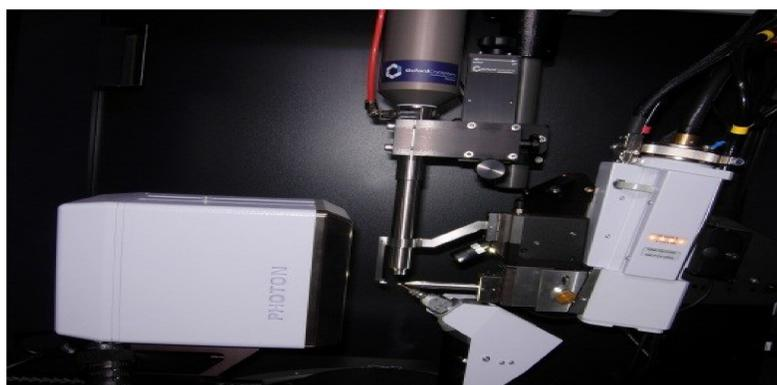
Samples are mounted on the tip of a thin glass or polymer fibre attached to a brass mounting pin, and the pin is then inserted into the goniometer head.
