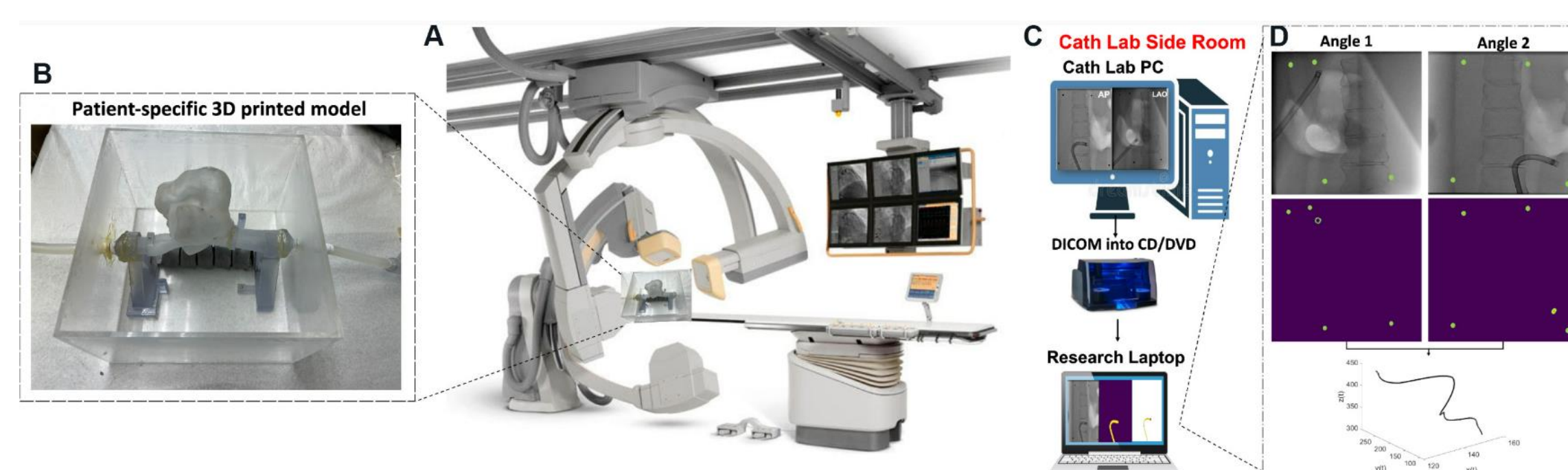
Figure 3. (A) Image of the 3D printed heart (B.) on a c-arm. (C) Scheme of the image transfer process of the post processed catheter tracking. (D) Image processing and deep learning steps of the fluoroscopy images.
