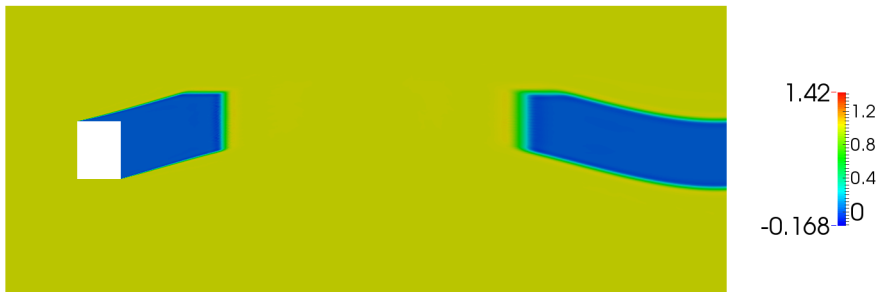
Figure 6: The approximations obtained using an SUPG method on an adaptively refined mesh containing 135,408,953 elements.
