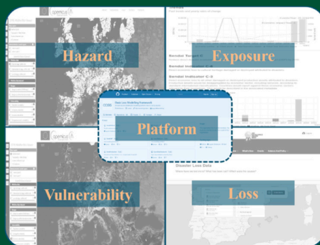
Figure 1: Insurance catastrophe models integrate regional and peril-specific hazard, exposure, vulnerability, and loss components to estimate expected loss
