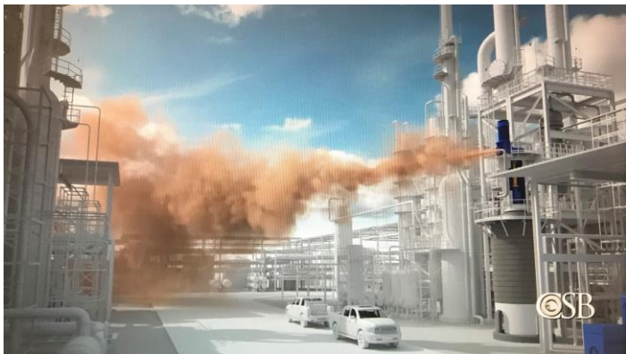
Figure 1: A computer-generated image depicting the horizontal release of ethylene vapour from EVAL Reactor 2's emergency pressure relief system. Image source: U.S. CSB
