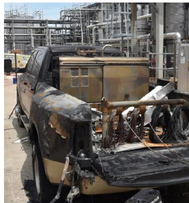
Figure 2: The welding machine on the back of the pickup truck, post-incident. Image source: U.S. CSB
