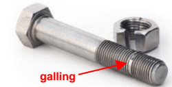
Figure 7: A bolt showing light thread galling after the seized nut was removed. Image not related to this incident. Image source: https://boltdepot.com
